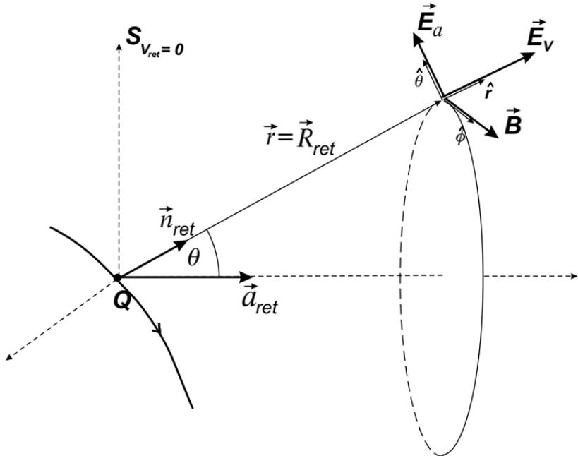
**Figure 1.** Spherical coordinates in the frame  $S_{V_{ret}=0}$ . At the retarded moment the source charge  $Q$  is at the origin of the frame and its retarded velocity is zero. As shown below, at the observation point the electric field has two components,  $\vec{E}_V$  along the radius vector and  $\vec{E}_a$  in the direction of  $\hat{\theta}$ . In turn, the magnetic field  $\vec{B}$  has only the  $\phi$ -component.
