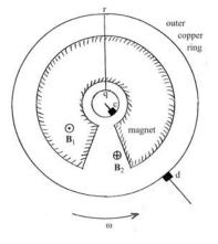
Figure 3. Generator Mode: Case A.
