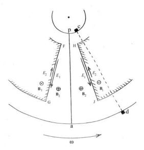
Figure 5. Induced electric fields in Case B.
