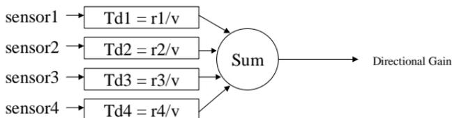
**Figure 2. Beamforming From Triangulation**
