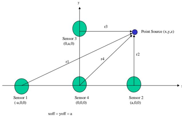
**Figure 1 Sensor Placement In The Array**
