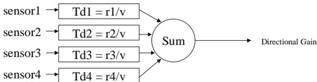
**Figure 2. Beamforming From Triangulation**
