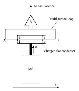
Fig. 8. Proposed scheme for an experimental test of SRT and LET.
