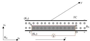
Fig. 3. An observer in the frame  $K_0$  sees that under motion of the frames  $K_1$  and  $K_2$ , the gray area ABDC decreases with time and hence, the magnetic flux across the conducting loop also decreases.
