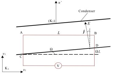
Fig. 5. Due to the Thomas-Wigner rotation between the frames  $K_1$  and  $K_2$ , an observer in  $K_1$  sees the space turn of condenser at the positive angle  $\Omega = uv/2c^2$ .
