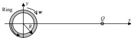
Fig. 10. Ring with the current I and charged particle Q initially rest in the laboratory. Then the ring begins to spin around the axis z at some constant angular frequency \omega . What is the force acting on the particle?
