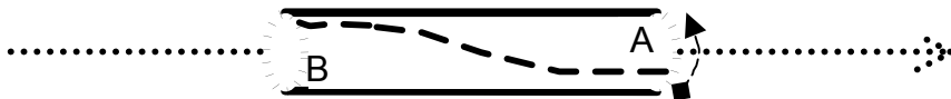
Figure 2. At any one instant, the observer will see a moving, rotating rod at progressively later times along its length from A to B. This makes the rod look shorter and its stripes appear twisted.
